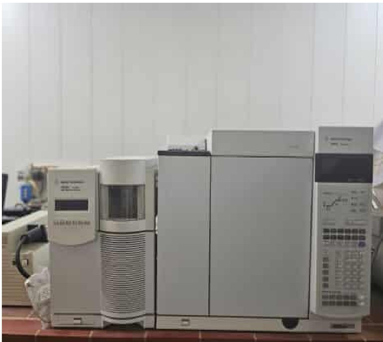
**GC system 7890A/5975C Inert MS with triple Axis Detector**
