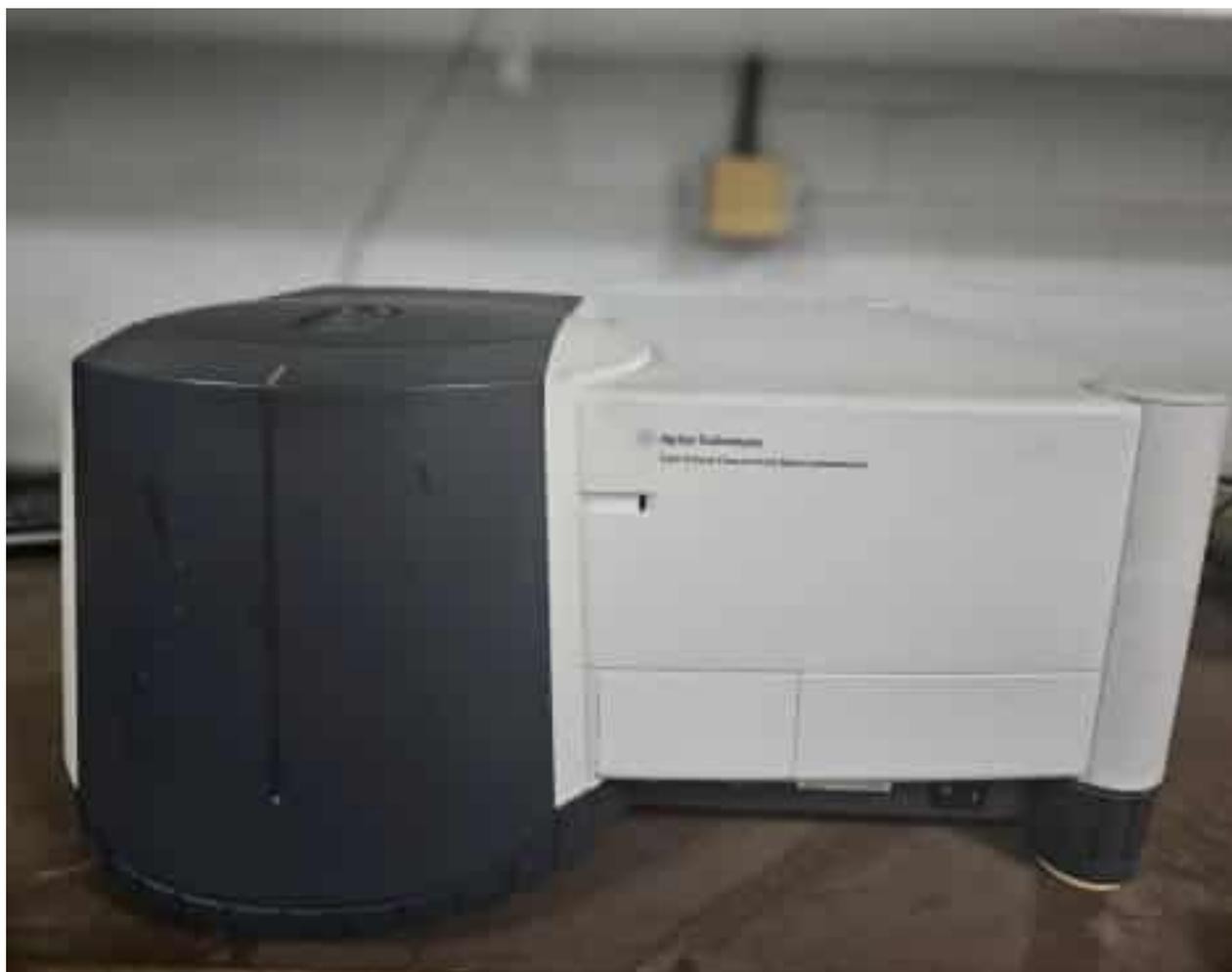
The Agilent Cary Eclipse is a fluorescence spectrophotometer. Fluorescence spectrophotometry is an analytical method used to measure the intensity of emitted light from a sample after exposure to excitation light. The Cary Eclipse is designed to provide high-performance fluorescence, phosphorescence, and chemi- and bioluminescence measurements
